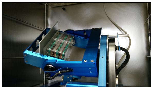
**Fig. 1.** Random Positioning Machine (RPM). The rotating frame of the desktop RPM was placed inside a CO<sub>2</sub> incubator for cell culture, and the movements of RPM were controlled by software through a specific algorithm. The culturing media were sealed with a transparent membrane, which was pressed to completely remove air bubbles from the culture chamber. Plates were placed beside the RPM machine so that all samples shared identical culture conditions.
